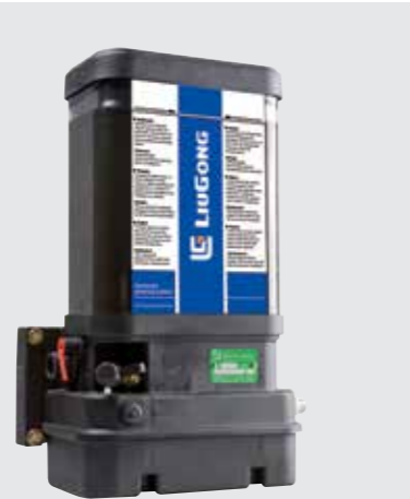
An automatic greasing system improves bearing life and reduces repairs by delivering regular and precise amounts of grease to each bearing.
